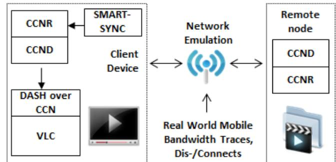
Figure 1. Demonstration Setup
